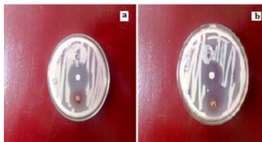
Fig. 6. Photograph of antimicrobial test results of Zn-ALG against a) S.aureus and b) E.coli
