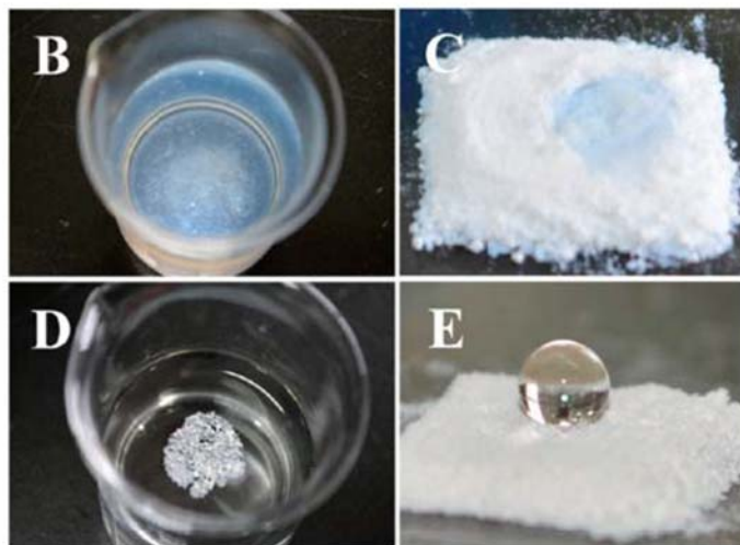
FIGURE 31.6 Image showing the comparison of surface wettability between silica (B & D) and OTS modified silica (C & E). Reprinted from Li X, Yu X, Cheng C, Deng L, Wang M, Wang X. Electrospun superhydrophobic organic/inorganic composite nanofibrous membranes for membrane distillation . 2015 http://10.1021/acsami.5b06509 copyright (2015) American Chemical Society.
